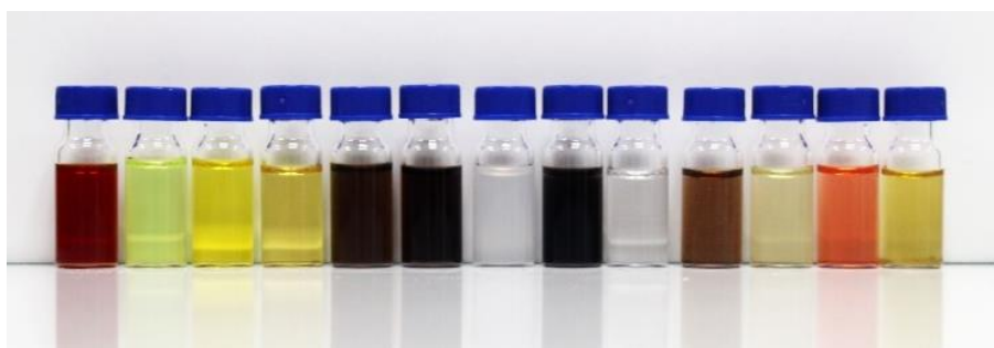
Supplementary Figure 2. Colloidal solutions of the all-inorganic NCs. From left to right: CdSe, CdZnSeS/ZnS, CdSe/ZnS, CdSe/CdS, PbS, \text{Fe}_2\text{O}_3 , \text{TiO}_2 , FePt, \text{NaYF}_4 , CdSe nanowires, CdSe nanoplatelets (wurtzite), CdSe nanoplatelets (zinc-blende), Ag NCs.
