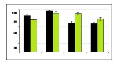
Fig.3. Removal of phenolic contaminants from actual samples (1-4) with selected AOPs  $(O_3/H_2O_2/UV \text{ (dark bars)})$  and  $O_3/UV \text{ (bright bars)})$ . For more information on the experiment, see Materials and Methods.
