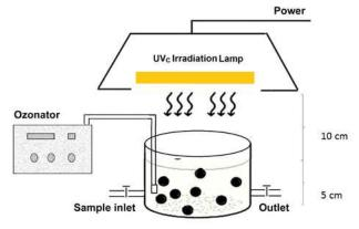
Fig. 1. Experimental arrangement for continuous ozone-based oxidation.
