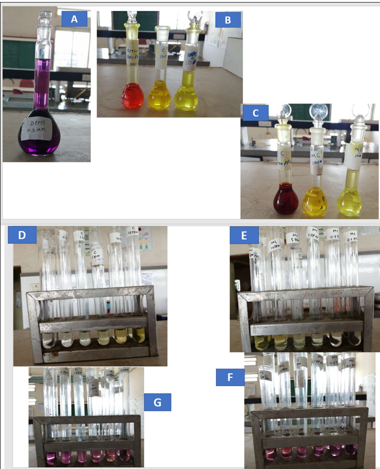
A: DPPH stock (0.2mM); B: Curcumin stocks(10,100,1000 ppm); C: Metal-curcumin complex(MCC) stocks(10,100,1000 ppm); D: Curcumin aliquots (before adding DPPH); E: MCC aliquots(before adding DPPH); F: MCC aliquots(after adding DPPH); G: Curcumin aliquots (after adding DPPH)
