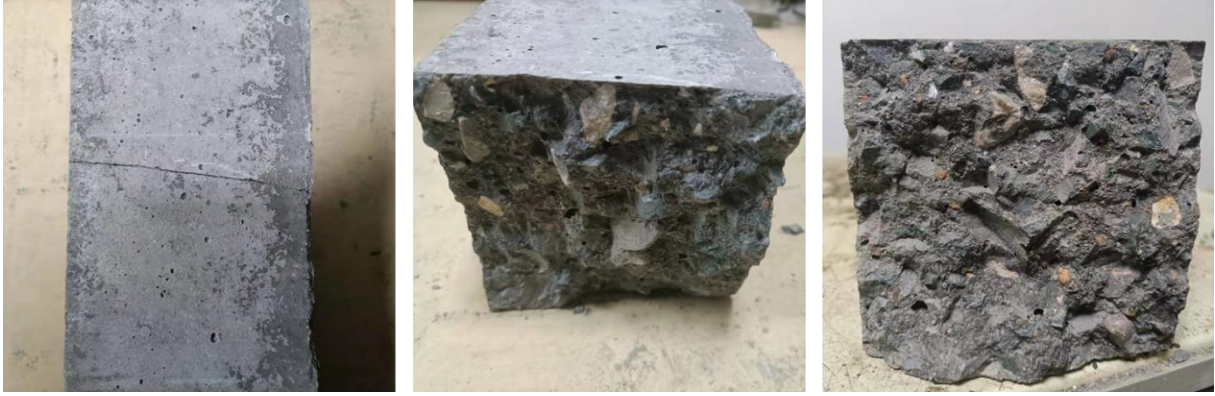
D: Flexural failure mode for PPMS and PPDG concrete
