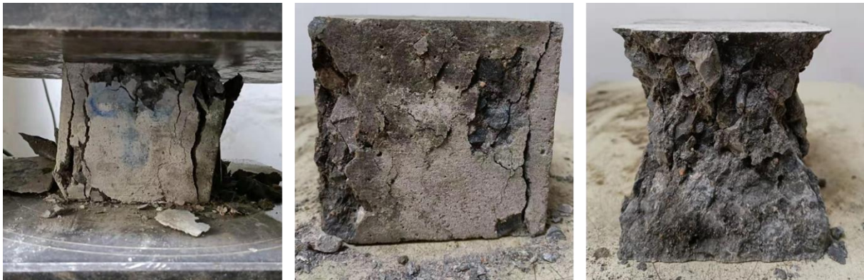
C: Compressive failure mode for PPMS and PPDG concrete
