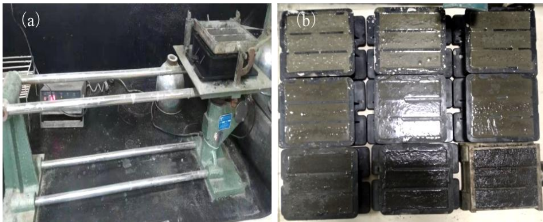
B: Wuxi Jianyi zs-15 cement mortar shaking table and cement mortar test block after shaking
