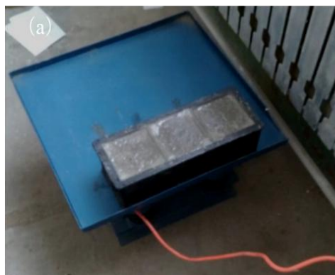
E: (a) Concrete shaking table (b) concrete test block without formwork removal
