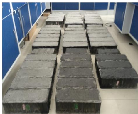
E: (a) Concrete shaking table (b) concrete test block without formwork removal
