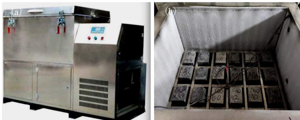
A: (a) Concrete freezing and thawing machine (b) concrete test block in frozen state
