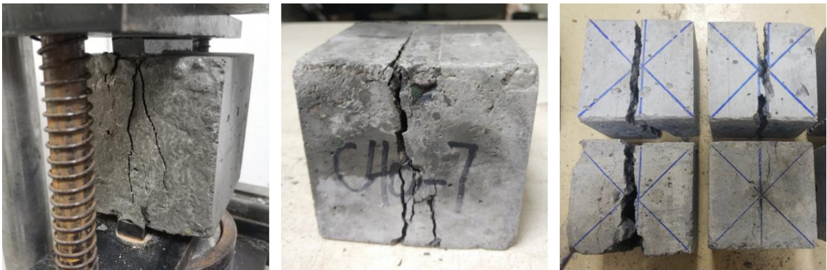
E: Mode of splitting tensile failure for PPMS and PPDG concrete
