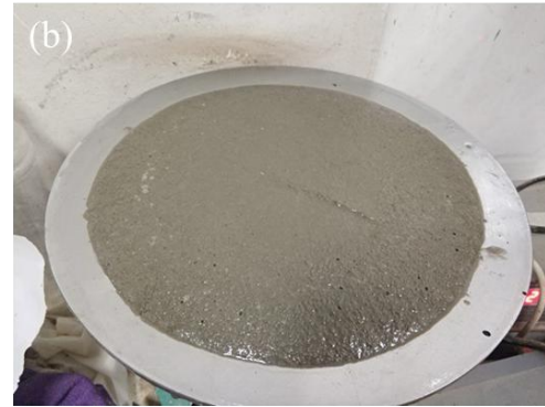
C: (a) Truncated cone circular die; (b) Table jumping to test fluidity
