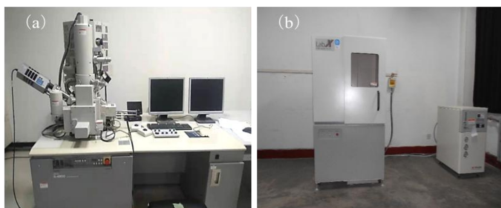
B: (a) Hitachi s-4800 cold field emission scanning electron microscope (b) xrd-6000 X-ray diffractometer
