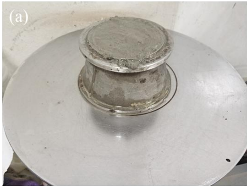
C: (a) Truncated cone circular die; (b) Table jumping to test fluidity
