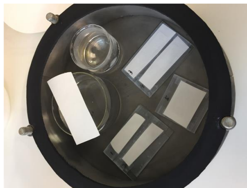
Fig. S1 the test assembly for investigating the water vapour-barrier property of the samples in harsh humid conditions: 20 °C, 95 % RH (provided by distilled water in the completely sealed container).
