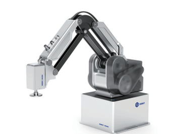
SI Figure 2. The specification for robots. a , the AUBO i5 robot; b , the DOBOT MG400 robot.
