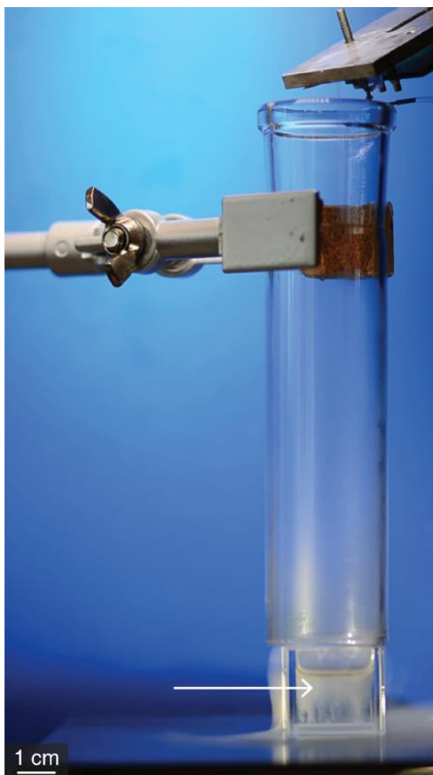
Figure S1: Photograph showing the emulsification achieved by separating the atomization unit from the oil bath with a 14 cm long glass tube. The arrow indicates the formation of the emulsion drops in the oil bath.
