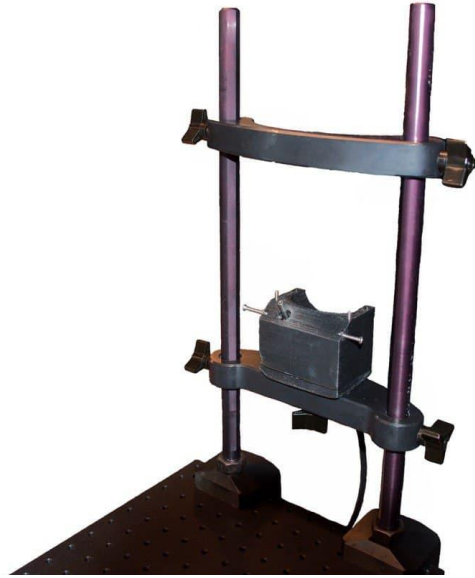
Fig. S13. Oral mucosa imaging setup, including a chin-head rest and a liquid light guide connected to a tabletop LED source for illumination. This photo shows how the liquid light guide is mounted in the chin rest.
