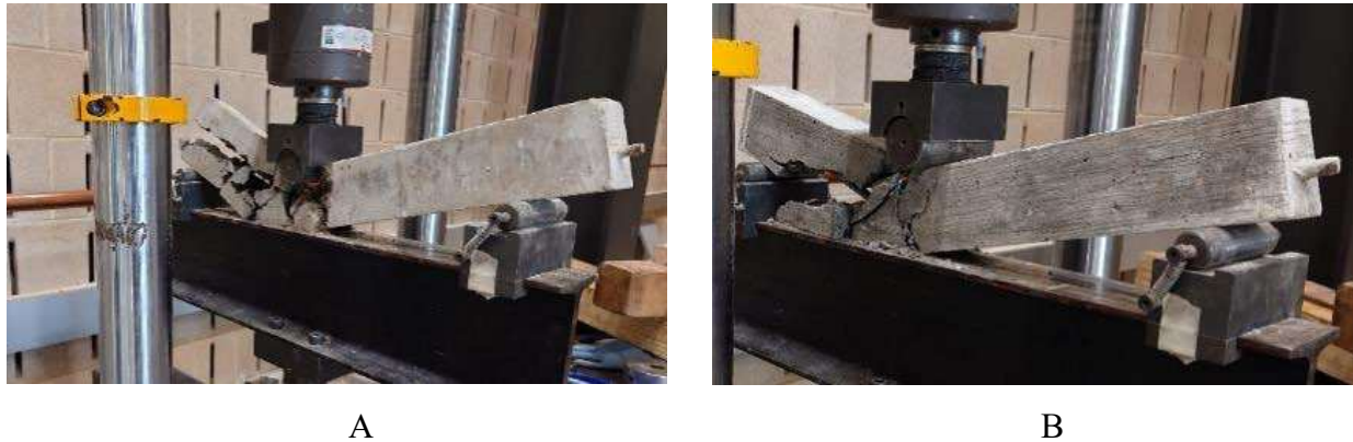
Figure 2. Center-point loading test on (A) carbon geocrete and (B) OPC concrete slender reinforced beams.
