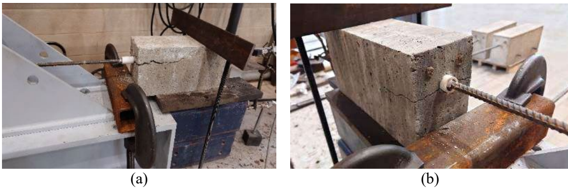
Figure 3. Bond strength testing on (A) carbon geocrete and (B) OPC concrete specimens conducted in accordance with ASTM A944 (ASTM International, 2023f).
