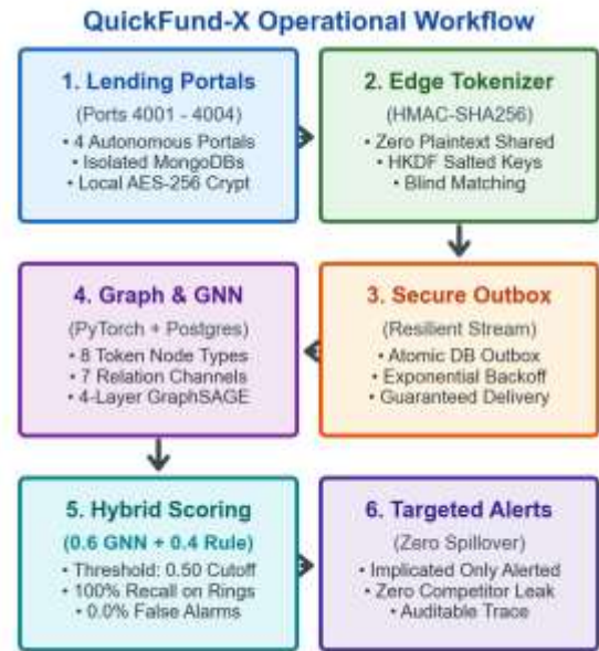
Fig. 1. End-to-end operational workflow of the proposed QuickFund-X cross-platform fraud intelligence architecture.
