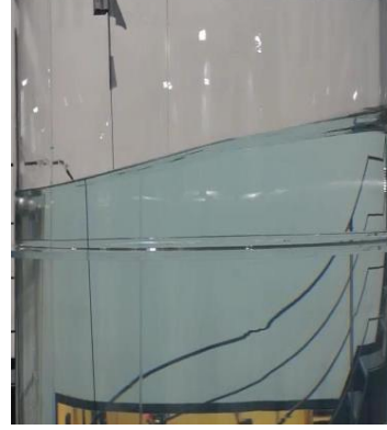
c) Our interIsoFoam sloshing model @4.9 s. d) Experiment by Konopka et al. [21] @4.9 s.
