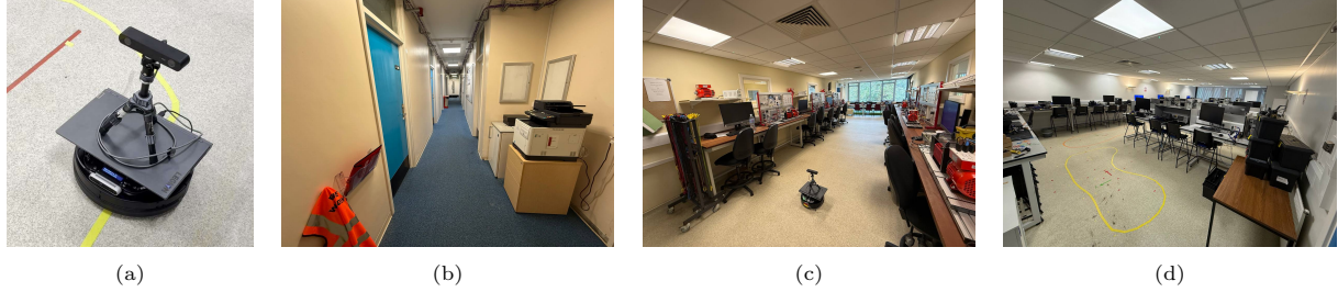
Fig. 2 Hardware platform and experimental environments: (a) a Kobuki mobile base carrying a ZED 2i stereo camera and a laptop; (b) the office area; (c) and (d) the laboratory area.
