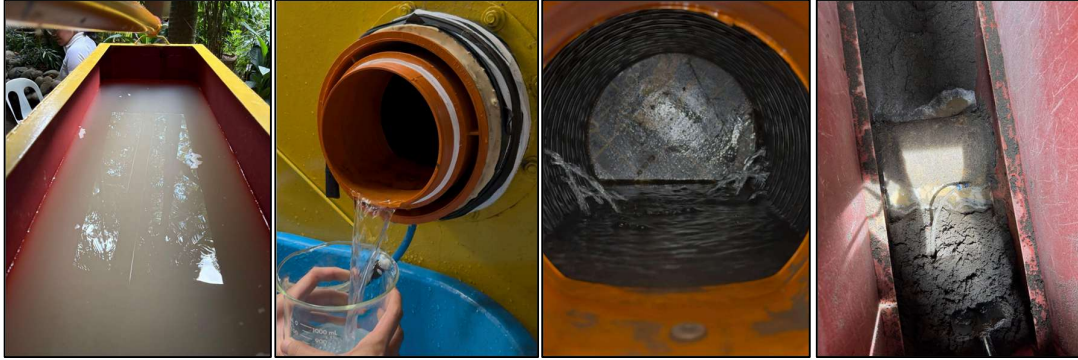
Figure 3. Soil tank experimentation. From left to right: Soil saturation, discharge measurement, in-pipe fluid flow in one-layer abaca geo-envelope, geotextile extraction.
