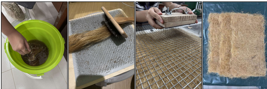
Figure 1. Abaca geotextile production. From left to right: NaOH soaking, carding board combing, needle punching, and finished non-woven abaca fiber geotextile
