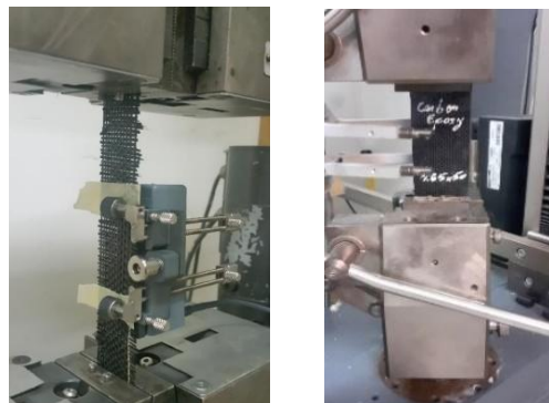
Figure 2. Tensile testing setup: (a) single-ply carbon composite laminates according to ASTM D3039 standard, (b) eight-ply carbon composite laminates.
