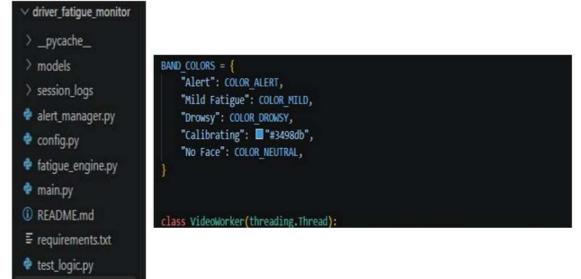
Fig. 3. Prototype project structure (left) and excerpt of the interface/worker code (right), showing the engine, configuration, alert-manager modules and the Alert / Mild Fatigue / Drowsy / Calibrating / No Face states.
