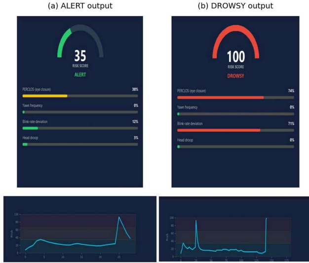
Fig. 7. Prototype dashboard output (cropped; webcam view omitted). (a) ALERT state, risk 35. (b) DROWSY state, risk 100. Qualitative demonstration.
