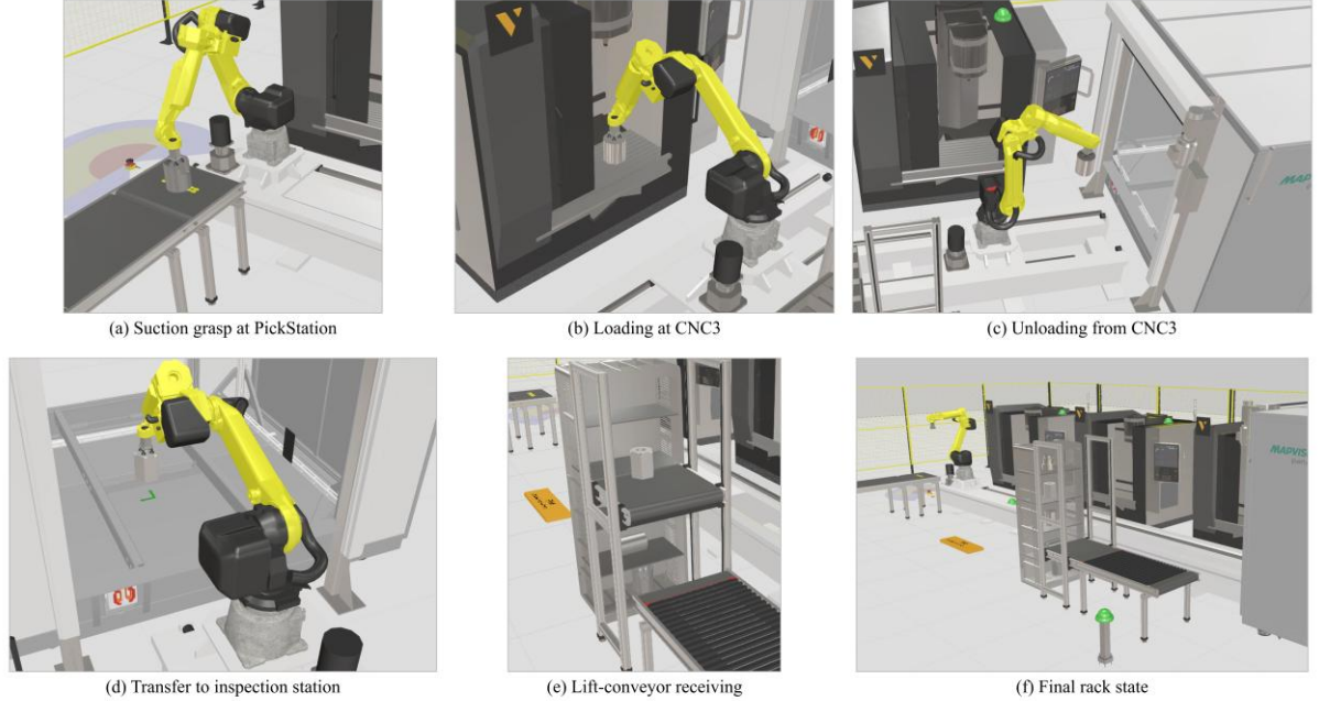
Fig. 8. Key frames of MIoT.VC virtual production-line execution validation.
