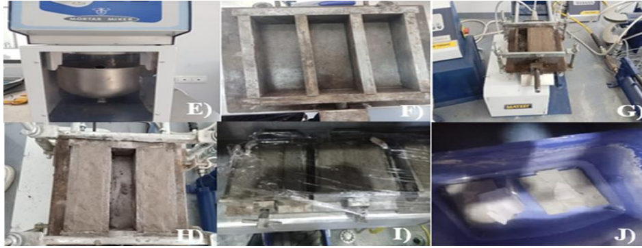
Fig 21. E) Mortar mixer, F) Mold samples 4×4×16 cm 3 G) Vibrating table to eliminate air H) Mold filled with mixture I) pockets in samples Cover in a damp room, J) The samples in the water.
