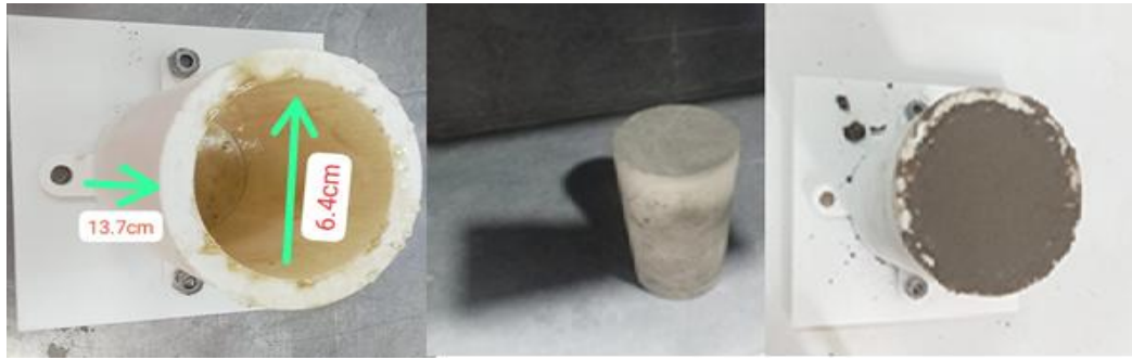
Fig 31. Mold and test specimen for shear testing
