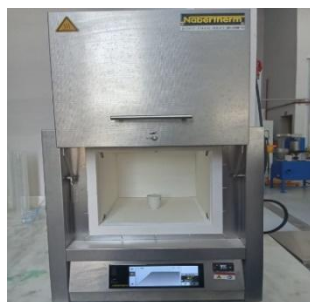
Figure 12. Glass filled in a muffle furnace (heated to 950C° for 3 hours)
