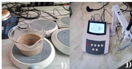
Fig 5. i) Agitation apparatus (sludge diluted in sterilized water) j). pH meter measurement
