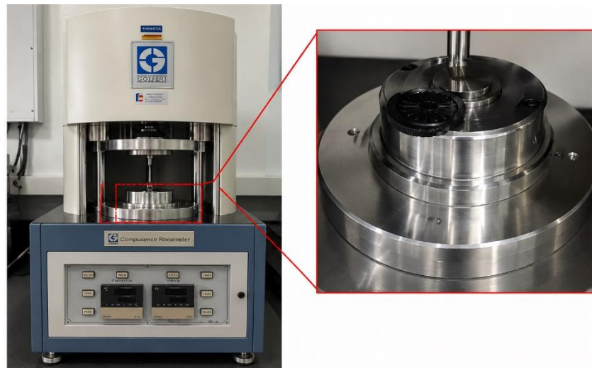
Figure 7. Moving-die rheometer setup for rubber curing characterization.
