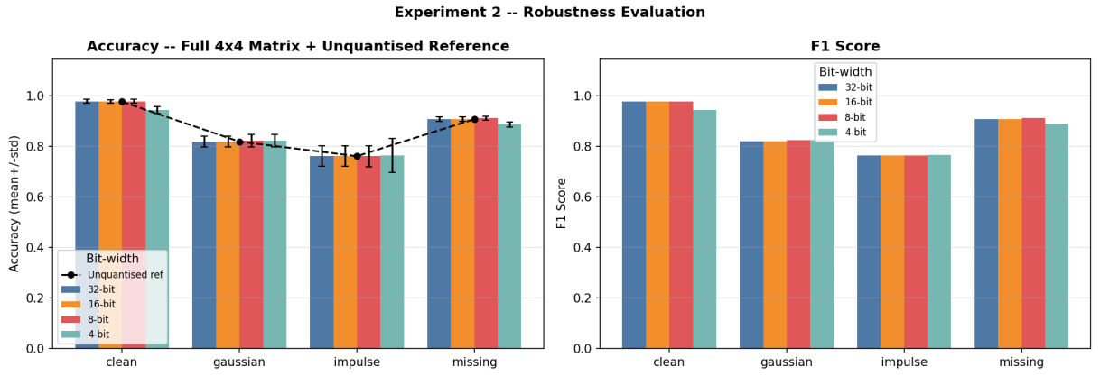
Figure 2. Accuracy and F1 for all 16 combinations + unquantised ref (dashed). Error bars=std, 5 seeds.
