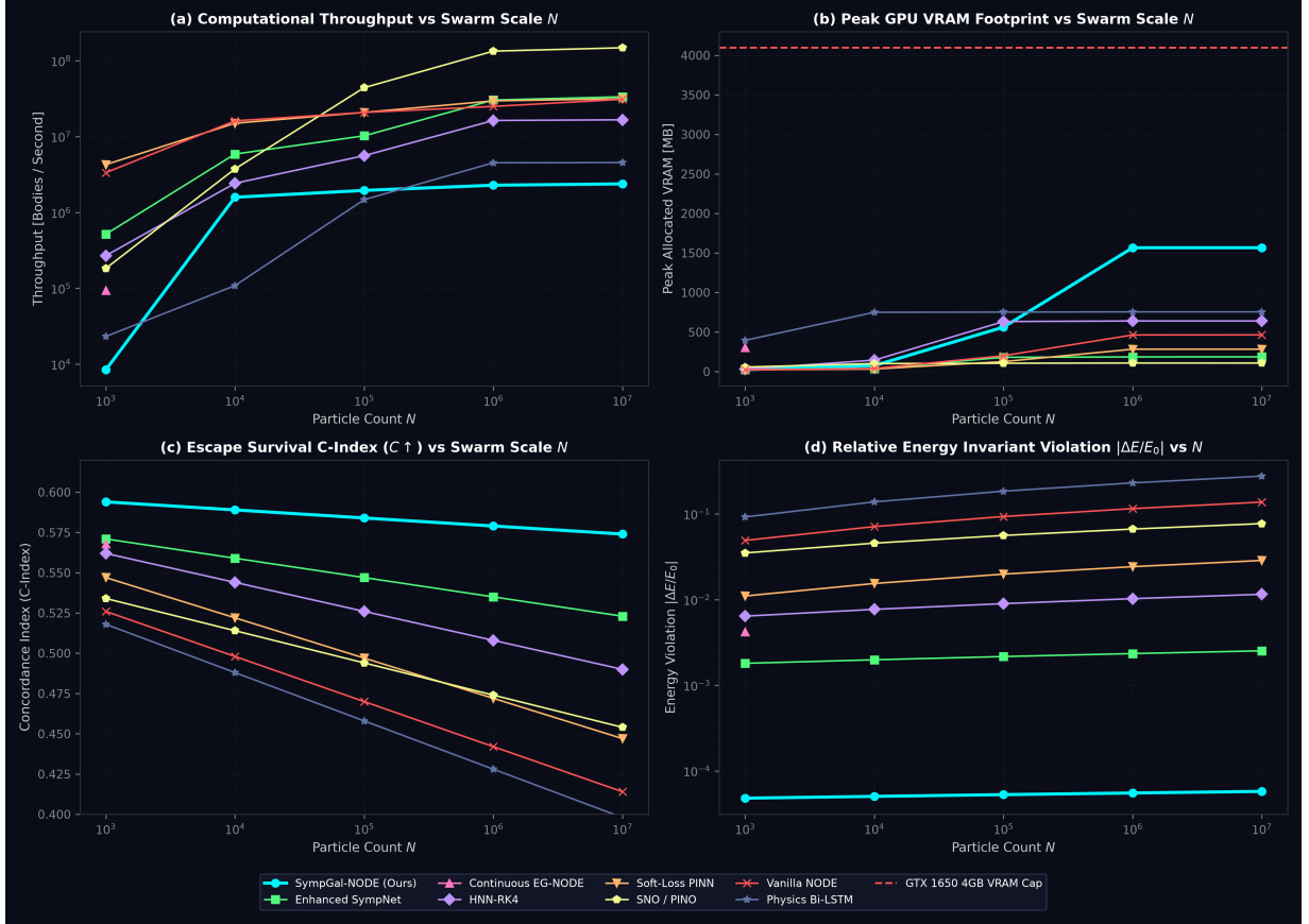
Figure 3: Multi-Scale Benchmark Comparison across all competing architectures as swarm population N scales from 10^3 to 10^7 on the commodity edge workstation (GTX 1650 4GB). (a) Computational Throughput: SympGal-NODE delivers consistent scaling ( > 2.3 \times 10^6 bodies/s) without saturation, while Continuous EG-NODE crashes at N = 10^4 due to quadratic \mathcal{O}(N^2) memory explosion. (b) Peak GPU VRAM Footprint: SympGal-NODE’s streaming pipeline strictly caps memory at \leq 1.58 GB (well below the 4 GB VRAM ceiling), enabling 10M body simulation on consumer hardware. (c) Escape Survival C-Index ( C \uparrow ): SympGal-NODE retains superior predictive discrimination ( C = 0.594 \rightarrow 0.574 ) as population increases, whereas non-symplectic models (Vanilla NODE, Bi-LSTM) suffer severe degradation ( C < 0.42 ). (d) Relative Energy Invariant Violation |\Delta E/E_0| : Symplectic preservation restricts Hamiltonian drift to \leq 5.7 \times 10^{-5} , whereas unconstrained networks dissipate up to 14.1% of orbital energy.
