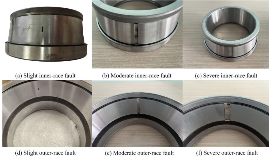
Figure 10. Schematic illustrations of bearing fault types.
