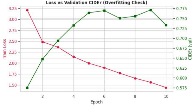
Fig. 11 Training diagnostics — overfitting check: training loss (left axis) decreases monotonically, while validation CIDEr (right axis) rises to a peak near epoch 9 and then plateaus, marking the onset of mild overfitting. This motivates the selection of the epoch-9 checkpoint as the cross-entropy model carried into the fine-tuning stage.
