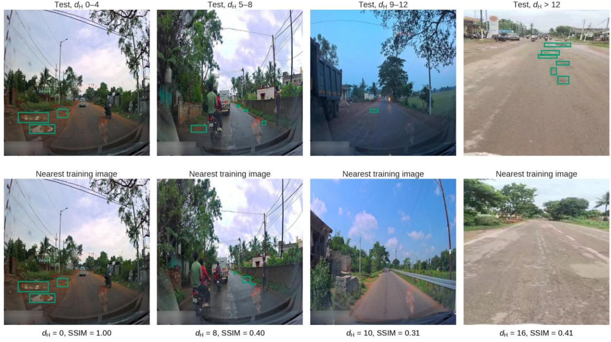
Fig. 3 One positive test image of the published split per d_H range (top) and its nearest training image (bottom). Green boxes: ground truth. d_H : Hamming distance between perceptual hashes; SSIM computed on 128 \times 128 grey thumbnails
