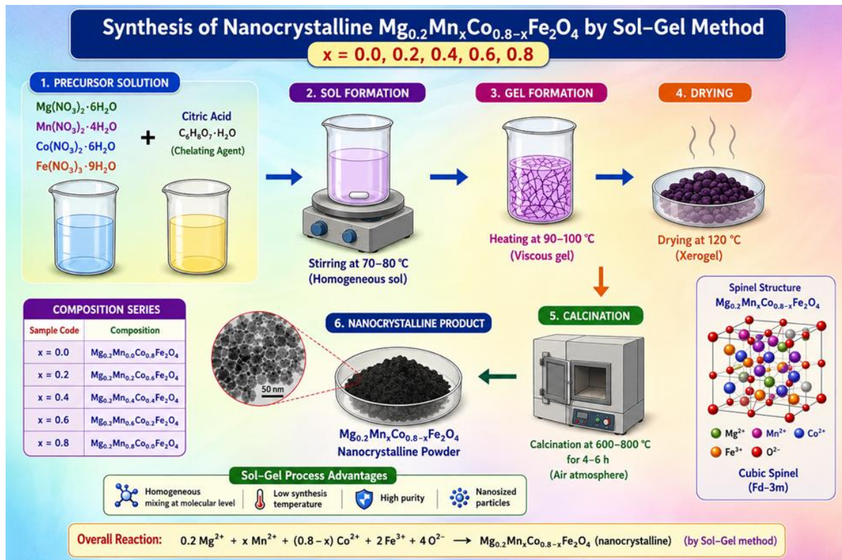
Figure:1. Schematic illustration of the sol–gel synthesis process for nanocrystalline A series of \text{Mg}_{0.2}\text{Mn}_x\text{Co}_{0.8-x}\text{Fe}_2\text{O}_4 (where x=0.0, 0.2, 0.4, 0.6 , and 0.8 ).
