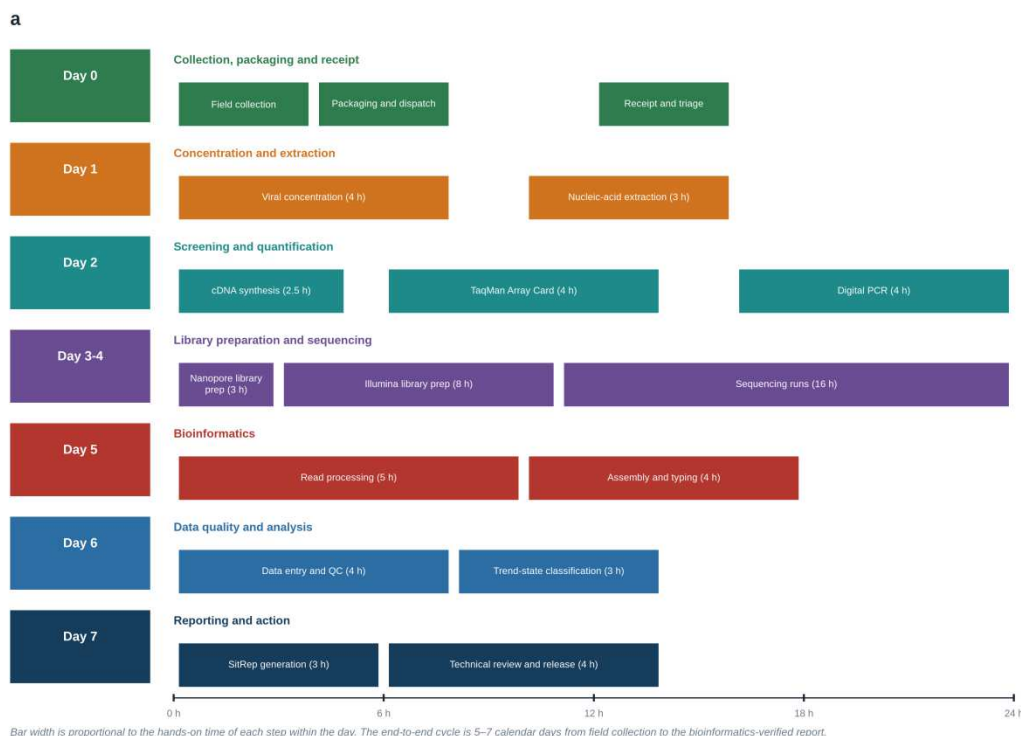
Figure 18: Per-cycle routine monthly WBE laboratory workflow - Day 0 (field collection and receipt) through concentration, extraction, TAC screening, dPCR quantification, and metagenomic sequencing to Day 7 (report).
