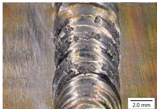
Figure 9. A typical plot of the current density changes with increasing temperature and a photograph of the root run of the weld on completion of the test showing the sites of pitting corrosion attack
