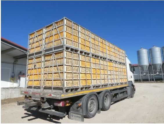
Figure 1. Transport vehicle and crate arrangement used in the two experimental batches. The vehicle was loaded with plastic transport crates arranged in 16 trolleys, with 8 or 10 crates stacked at different vertical levels.
