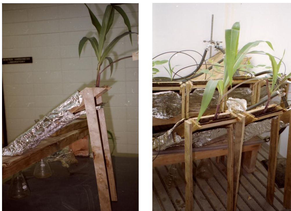
Fig.1. Corn grown in the rhizotrons positioned at a 45° angle on a stand and kept hydrated at the rhizotron capacity using trickle irrigation system.
