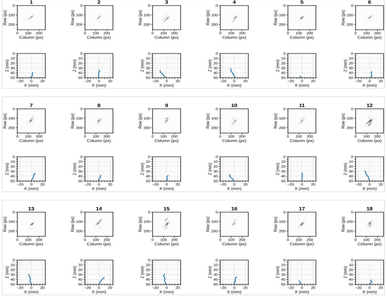
Figure 2. Representative simulated inspection responses and associated reference flaw contours. Each contour is represented by 11 ordered points, corresponding to a 22-coordinate regression target.
