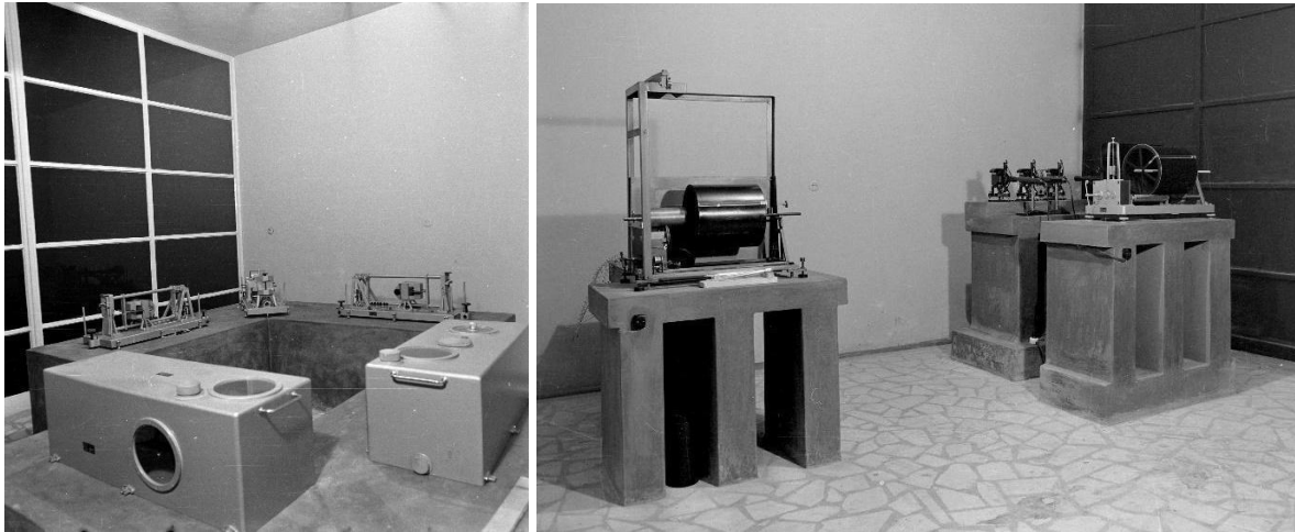
Figure 12. The electrodynamic seismographs SKD (Z, NS, EW components) installed at Timisoara station in 1970: The sensors ( left ) and the photographic recording system ( right ). Source: Photographic archive of the Timisoara Seismological Observatory
