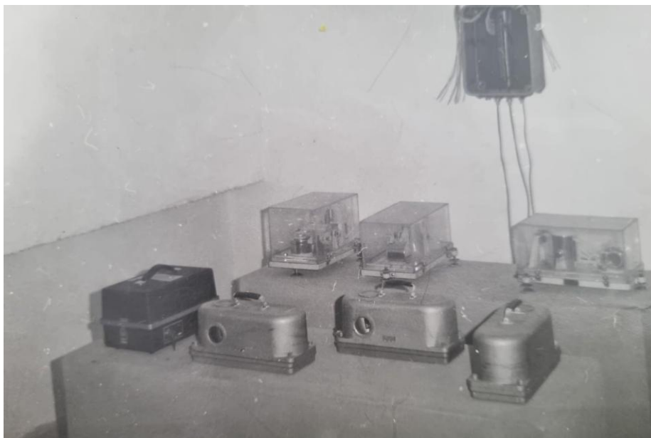
Figure 21. The 3 component DD1 seismometer (cased in plexiglass box) and of the S5S seismometer (cased in metal box) Source: Photo archive of the Timisoara Seismological Observatory
