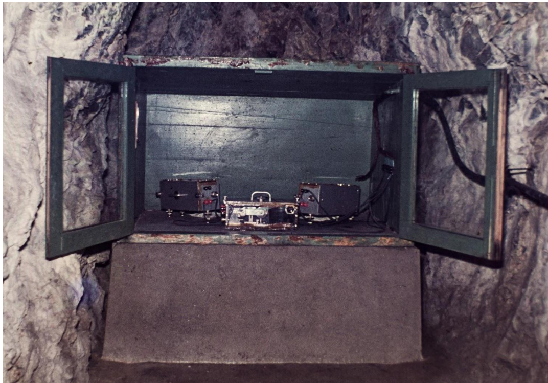
Figure 14. Vegik seismometer installed at Susara station in the early 1970s Source: Photographic archive of the Timisoara Seismological Observatory
