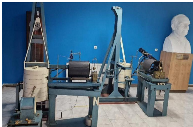
Figure 10. Mainka-Demetrescu-Curea mechanical seismographs installed at the Timisoara Observatory in 1966 ( left ); the same instrument in a preservation state in 2025 ( right ) Source: Photographic archive of the Timisoara Seismological Observatory
