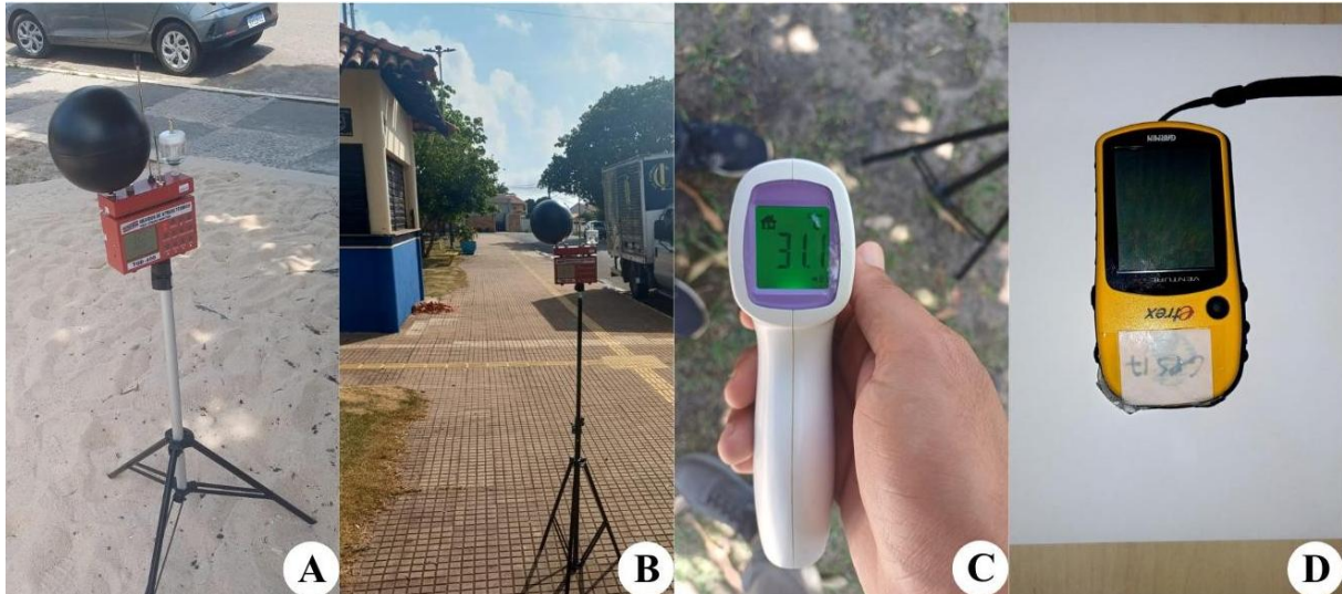
Figure 2. Equipment utilized for data collection. A - Heat Stress Meter: data collection in a tree-shaded environment. B - Heat Stress Meter: data collection in an unshaded environment. C - Infrared Thermometer. D - Garmin eTrex 10 GPS.
