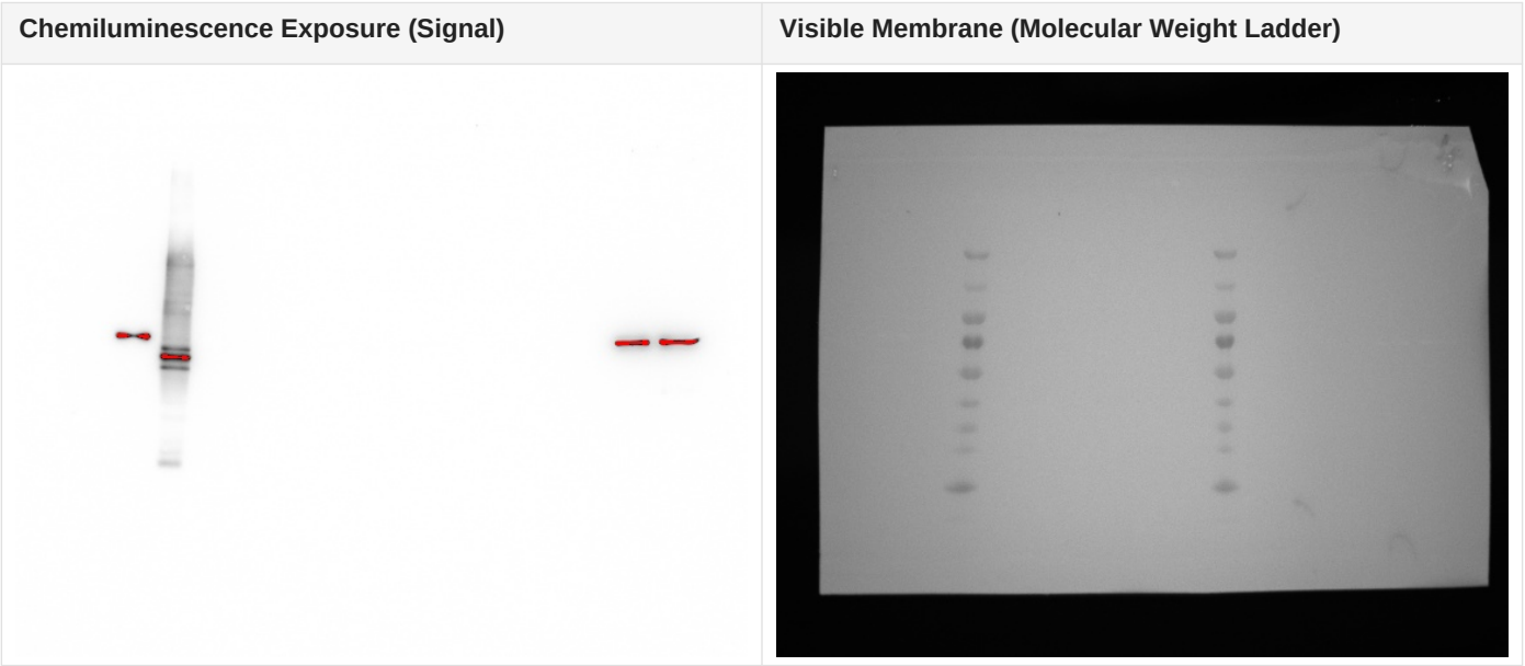
Panel Annotation Notes: Prestained molecular weight ladder (L) positions correspond to 170, 130, 95, 72, 55, 43, 34, 26, and 17 kDa. C57BL/6NJ control and PS19NJ transgenic age series: 13, 19, 26, 32, and 39/40 weeks. The red box on the cropped manuscript figures corresponds to the main immunoreactive band(s) visible in these full-length captures.
