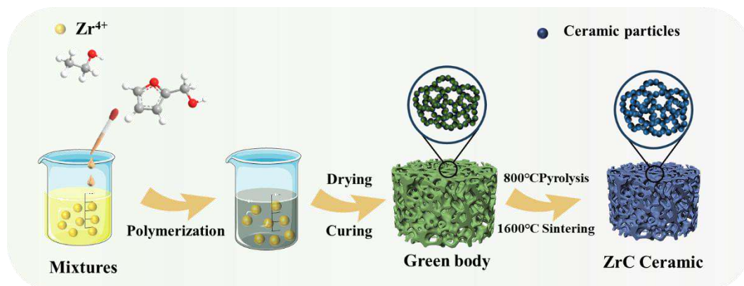
Figure 1 Schematic diagram of the preparation process for ZrC porous ce-ramic.
