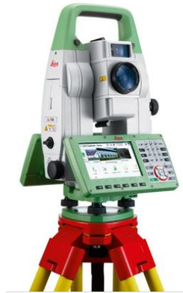
Fig. 1. A high-precision Leica TS16P1R500 Total Station used in the study
