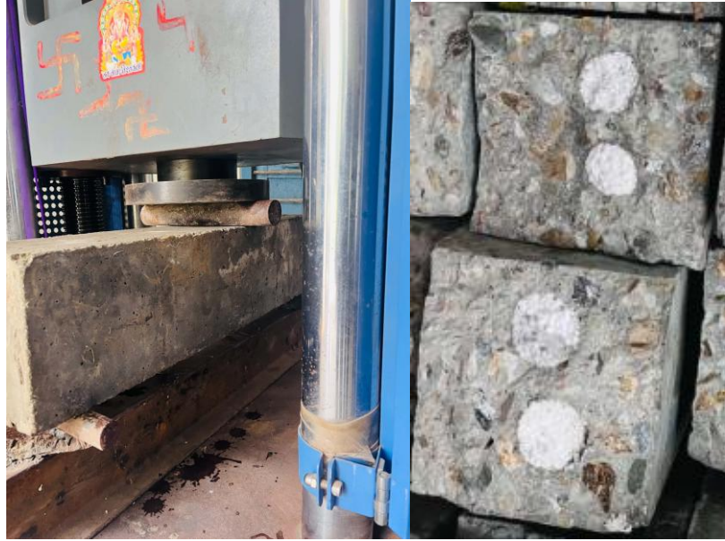
Fig. 6: Three-point flexural strength testing of beam specimen during and after the test.
