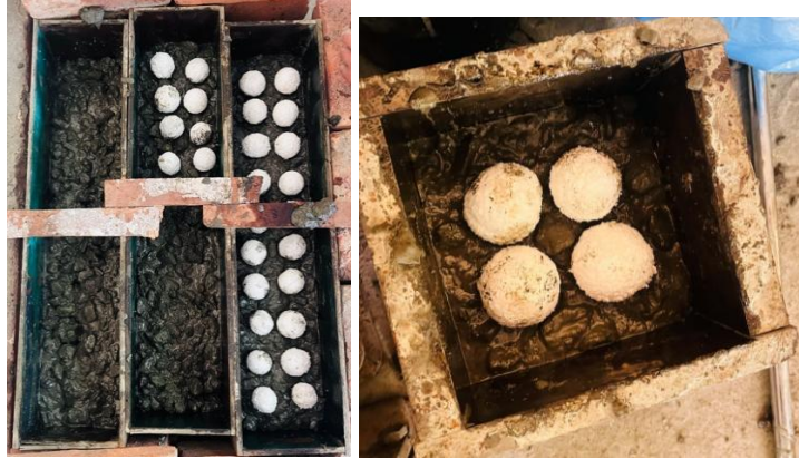
Fig. 4: Thermocol placement at the core of the Beam and cube
