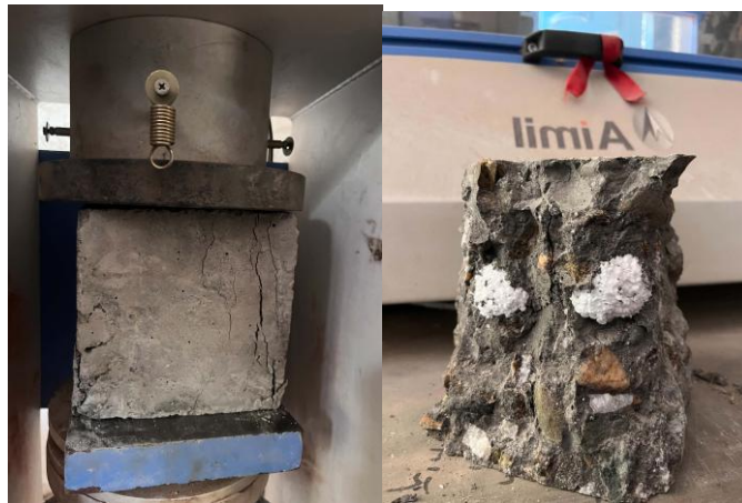
Fig. 5: Compressive strength testing of cube specimens during and after the test.
