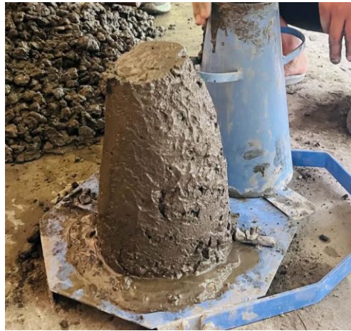
Fig. 3: Slump cone test on fresh concrete.
