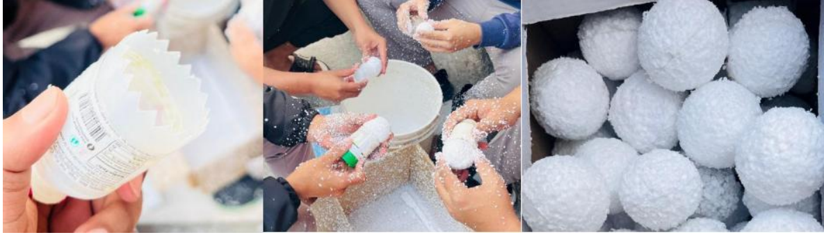
Fig. 2: Fabrication of spherical Thermocol core formers: shaping the half-cut-bottle jig (left) and sanding cubical blanks into uniform spheres (right).
