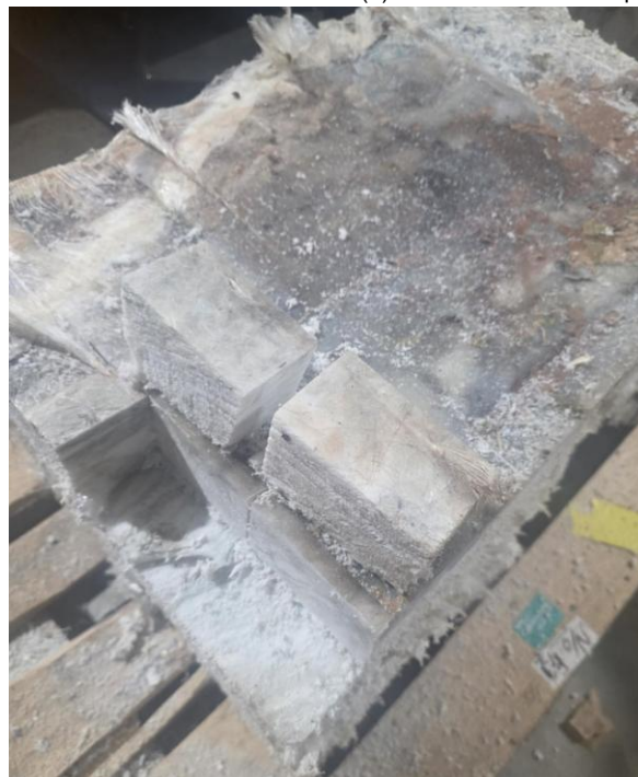
(e) Sections cut from consolidated heterogeneous material
