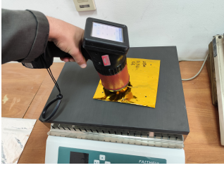
Fig. 12: MLI's emissivity measurement using the ET10 reflectometer.
