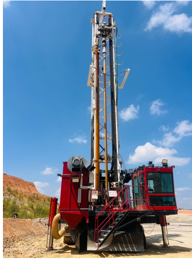
Fig. 7 ZY250E intelligent tricone rotary drill rig used in field tests
