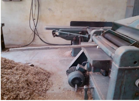
Figure 5a: Surface planing of the cured engineered bamboo beams.
