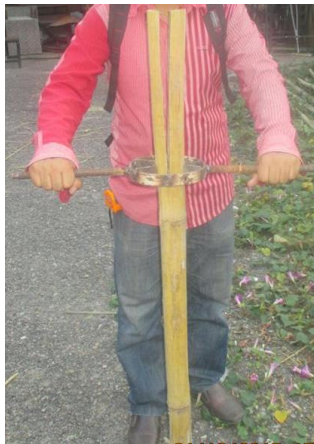
Figure 1a: Mechanical splitting of bamboo culms into longitudinal strips.
