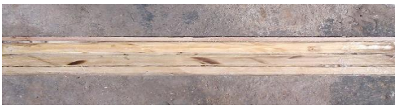
Figure 5b: Final processed engineered bamboo beam ready for mechanical testing.
