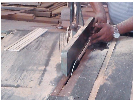
Figure 1b: Removal of pith and skin layers and strip sizing using a table saw.
