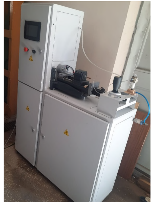
Figure 1. Experimental test setup (1- Housing, 2- Panel Screen, 3- Fixed bed, 4- Nozzle, 5- Powder tank, 6- Powder supply line)
