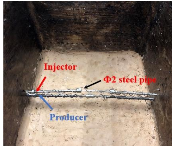
Fig. 7. Preheating tubing around the horizontal well pair.
