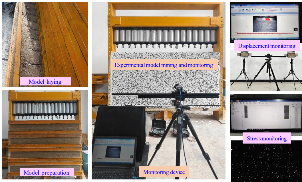
Fig. 4. Physical analog model (PAM) and modeling process.
