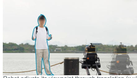
Robot adjusts its viewpoint through translation (x,y) and rotation (yaw, pitch)
