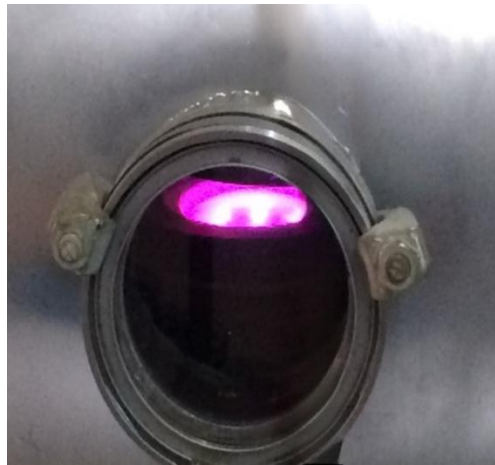
Figure-3. Plasma formation during the plasma-sputtering process.
