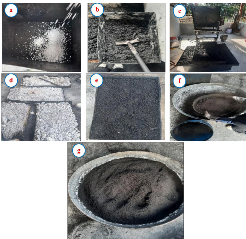
Fig. 1 Steps in the production of genetically modified porous carbon in a thermal furnace: Mixing the initial biochar with activator and water (a, b), placing it inside the furnace (c), porous carbon from tissue paper waste (d), straw (e), grinding and sieving the product (f), final product (g)
