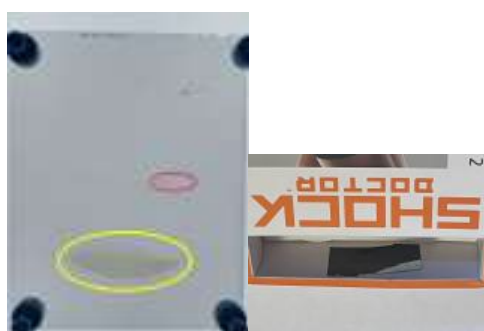
Figure 12. An explanation was found for a light leak (encircled in yellow) on the monitor film in the 4 th position. A piece of tape used to cover a manual hole in the box containing the culture plate and film assembly was partially lifted. Even though the tape was still on, a slight lifting was enough to result in a noticeable exposure of the high-speed film after 36 hours.
