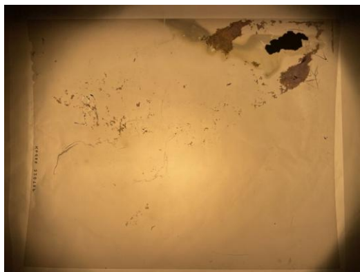
Figure 9. Film contaminated with graphite after sticking to the barrier layer.
