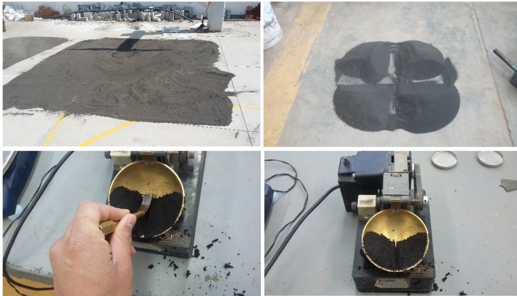
Figure 3. Index properties were determined following standard geotechnical procedures, including: natural moisture content, grain-size distribution, specific gravity of solids, and soil unit weights 1
