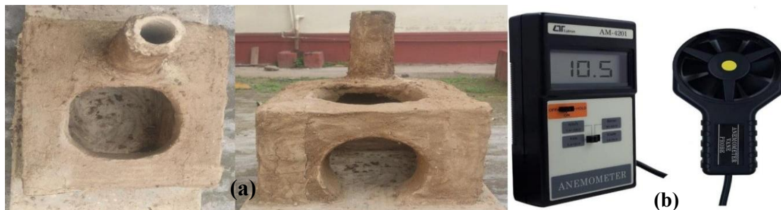
Figure-3 (a) picture of original chulha, (b) Anemometer
