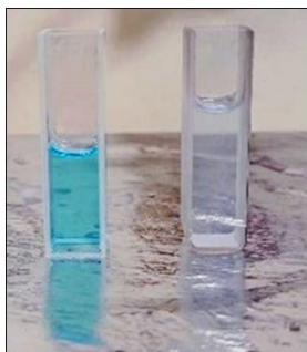
Figure 13(c) The appearance of methylene blue before and after photo gradation under UV irradiation after one hour duration
