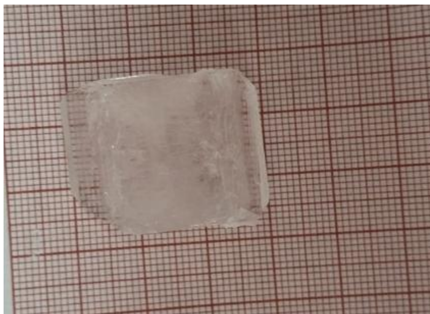
Fig1. As-grown (LPSN) single crystal
